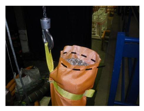
3) When the tube is adequately filled, seal the end using the attached string / tie wrap:
